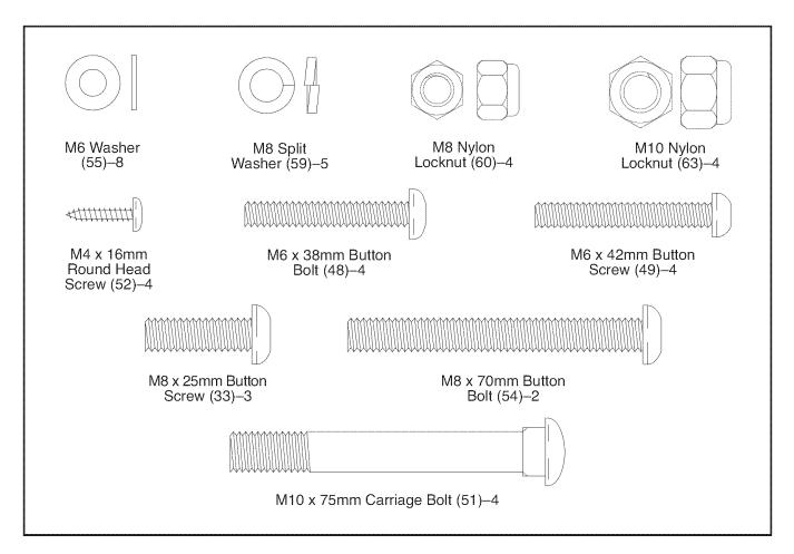
1. While another person lifts the front of the Frame (1) slightly, attach the Front Stabilizer (3) to the Frame with two M10 x 75mm Carriage Bolts (51) and two M10 Nylon Locknuts (63).
